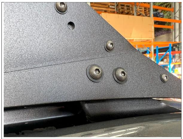
133. Lower rack back down and secure Rack to L Brackets with 2x M8x20 Button head bolts and M8 Flat Washers Per Side
