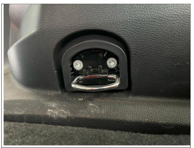
53. On the RHS Only remove the tie down point from the side of the cargo area by removing the 2x T30 Countersunk Screws
