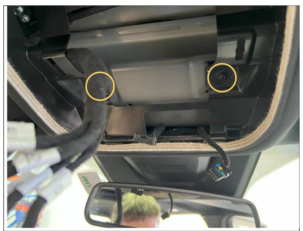
41. Using a T20 Torx bit, remove 2 screws shown securing the plastic roof liner support to the roof.
