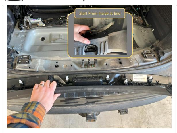
52. Remove the rear step trim, pull firmly from the inside upward, starting at each end to progressively release clips.
