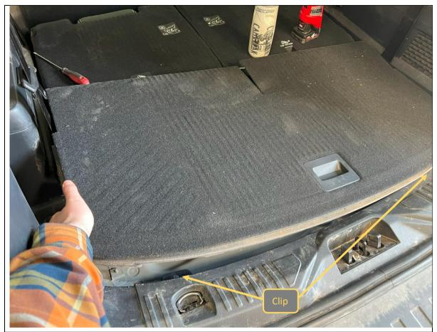
51. Release the 2x Clips securing the Jack/Tool Storage area tray to the rear trim and lift out the Jack/Tool Storage area tray.
