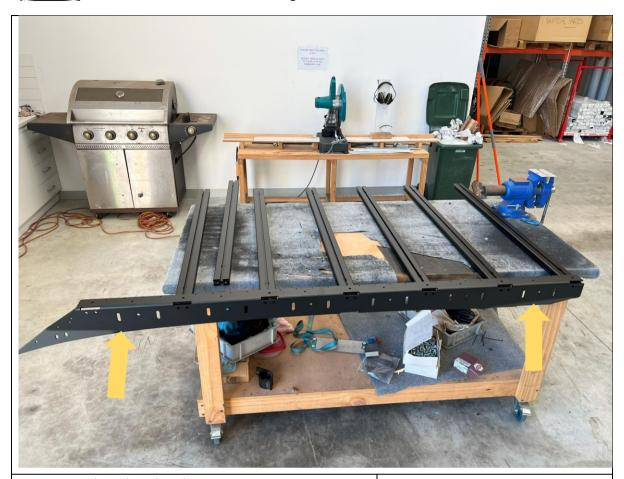
2. Fit the side rail to the extrusion,
