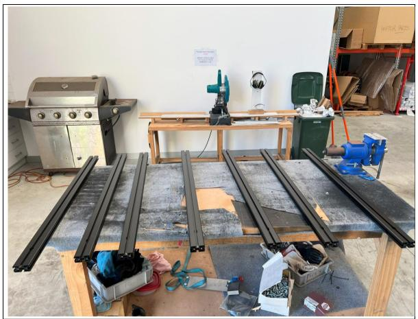
First thing is to Assemble the roof rack. Start by setting out the 7 extrusions on a table. Position them so they sit approximately 200mm apart.
