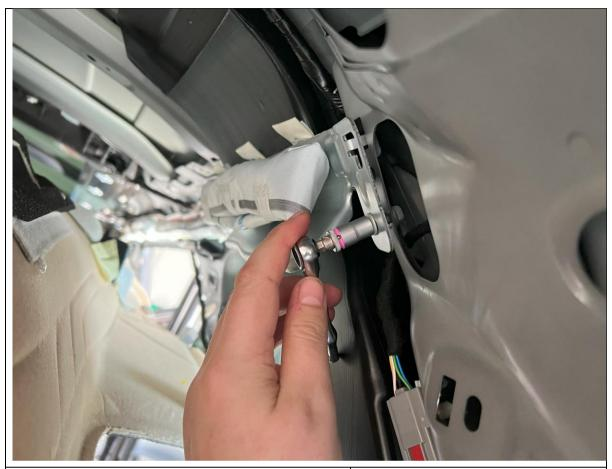
86. Using 8mm Socket, remove the rear bolt securing the air bag support bracket, and loosen the front bolt. Let the bracket hang down slightly, being careful not to let the airbag crease significantly.
