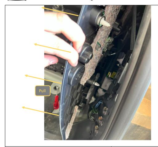
60. On the RHS Only remove the Lower side cargo area trim panel. Start by pulling away from body near the rear tailgate rubber to start releasing clips.
