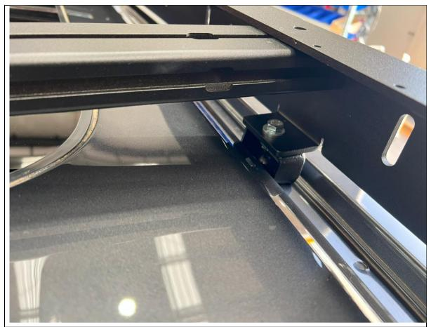
136. Secure the rack to mid mounts using M8x20 Hex Bolt and washer into the pre-fitted Cage nut.
