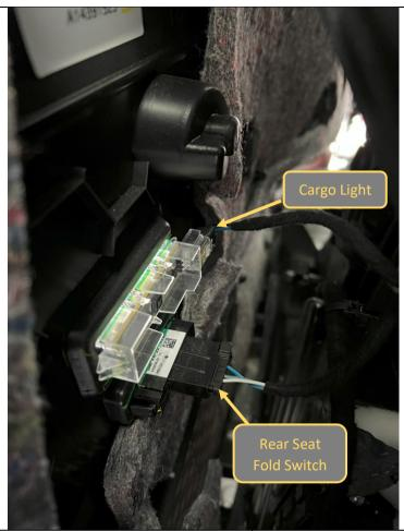
61. Once enough clips are released for access, unplug the cargo light and rear seat fold switches (if equipped).
